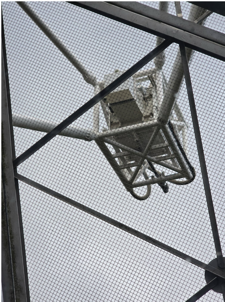
Fig. 2. View through the control-room skylight showing the 25-meter wire-mesh reflector and the feed assembly at the prime focus. The mesh size is 8 mm, allowing the dish to operate from a few centimeters to a few meters in wavelength.
