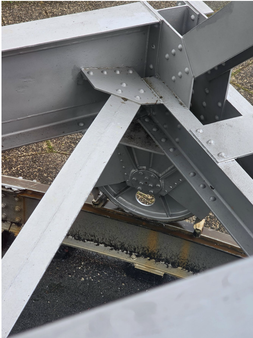
Fig. 1. Wheel carriage running on the circular track at the base of the 90,000 kg structure. Brushes on either side of the wheel sweep debris from the rail before each rotation. Every startup requires a careful walk-around inspection.
